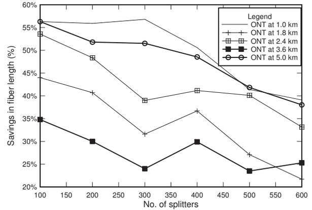
Figure 4. No. of splitters versus fiber savings.
