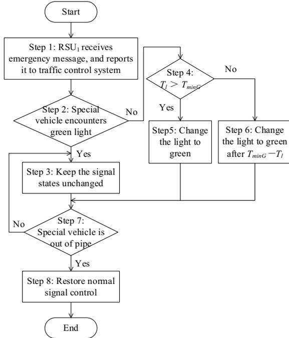
Fig. 4 The process of adjusting signal phases
