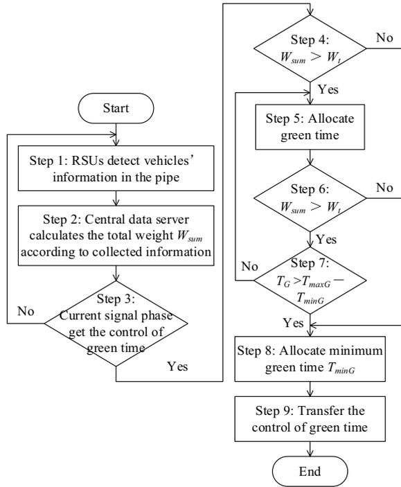
Fig. 3 The process of allocating green time
